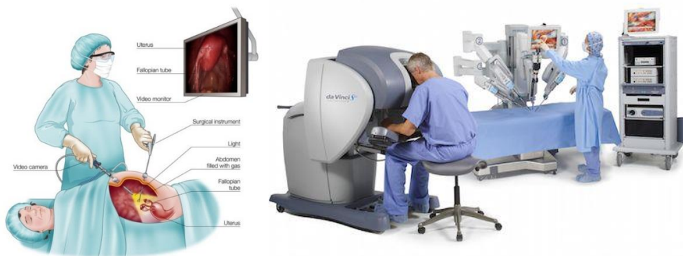
Fig. 8 Traditional laparoscopic surgery setup (left) [71] vs. Robotic-Assisted MIS surgery (right) [72]
