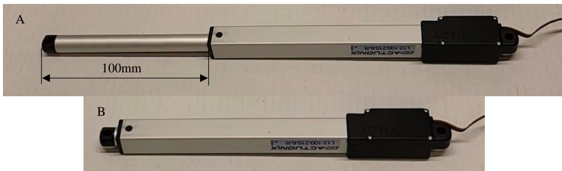
Fig. 41 Linear micro servomotor (L12-R manufactured by Actuanix®)
